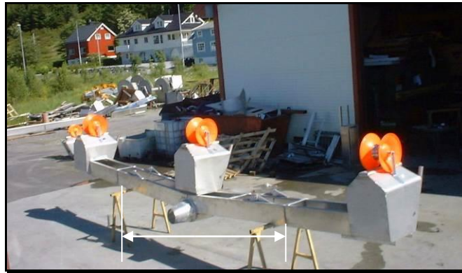
Picture 5 Standard system aft with 3 receivers on conveyor chute, rollers and a tract in the middle
