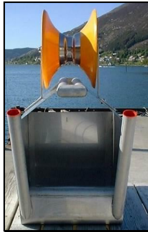
Picture 1 "Fish receiver" which unhooks the fish from the line
